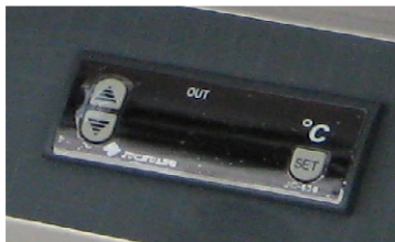
1. Manual temperature adjustment for the best control of chocolate's viscosity (Range: Room - 45°C)
